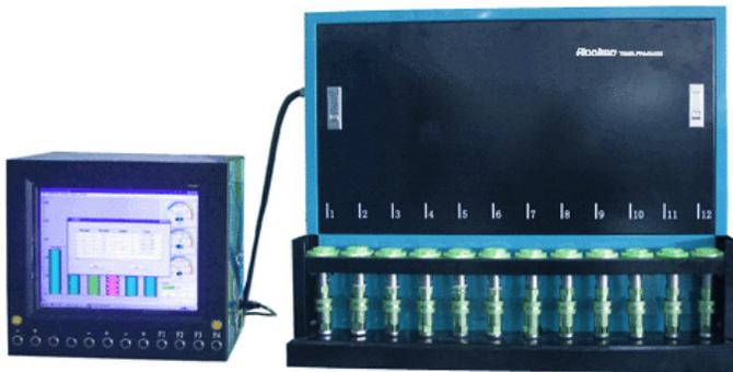
Model **RTEFC12** is a computerized fuel measuring and collection system with separated graphic display/indicators for up to 12 injectors (cylinders). This is an add-on kit designed to replace the traditional glass graduate tubes and can be attached on any models of Rocken Tech test stands.
