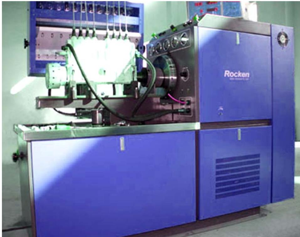
Rocken Tech test benches are available in 7.5kW (10hp), 11kW (15hp) and 15kW (20hp), 18.5kW (25ph), 22kW (30hp) and 37kW (50hp). They have been recognized in compliance with the ISO 4008, ISO9001 and 2000 regulations for testing and calibrating in line and rotary diesel fuel injection pumps.
