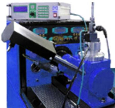
This simulator is designed to test the functionality of UPS injection pumps (Unit Pump System) and Injectors-Pump (EUI). It is composed by two units:
